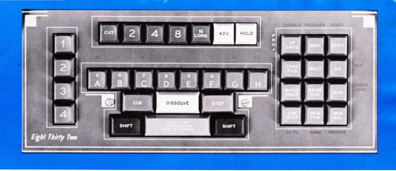
For fancy animation or sequence repetition, the 800 allows DO-NEXT LOOPS. One can specify up to 99 repetitions of a sequence beginning with the DO command and ending with the NEXT command . . . **three simple steps.** Loops may be NESTED four deep and can be used with any type of program entry.
