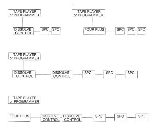
In all of these examples, you will note that the SPCs are not connected between the other models, but are in the trailing position of the hook-up.
